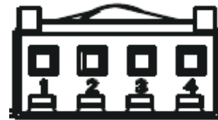
Fig. 13 – Sensor Wire Harness Pin Layout
